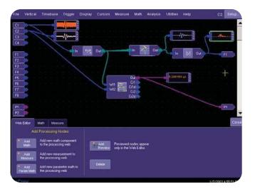
With the XMAP option, LeCroy's Processing Web lets you think about signal analysis graphically. Visualize an oscilloscope measurement as a chain of operations while seeing results at every step.
